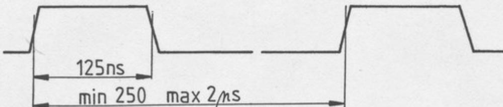
7. CPU 80286-8 Reset input (IC2 pin 12): low level
