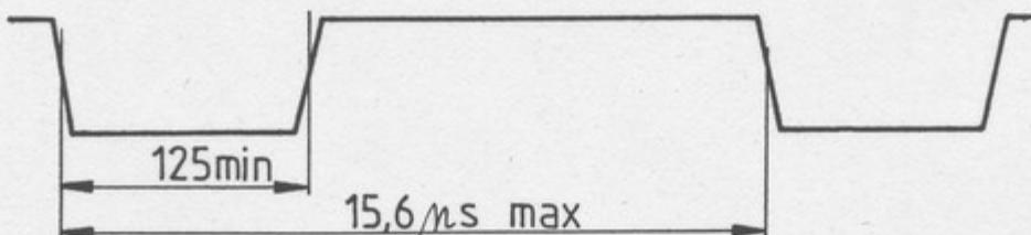
12. MUX (IC68 pin 12): high level
